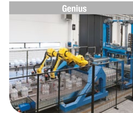
Genius Complete traditional palletising and depalletising systems, with high and low feeding.
