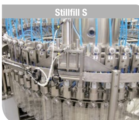
Stillfill S Gravity mechanical filler suitable to cold fill still water and not carbonated products.
