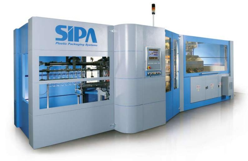
**Preform transfer.** After heating, preforms leave the oven and are transferred to the blow moulding station by means of a variable pitch unit operated by a servo motor.
